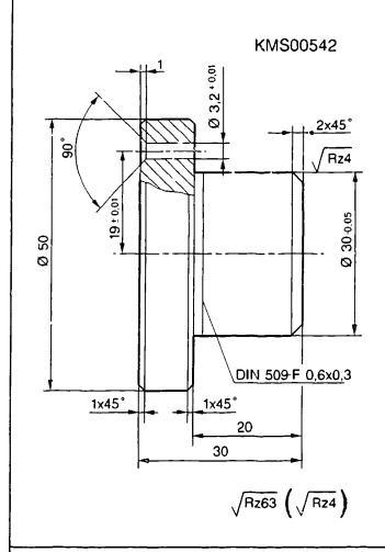
Tool for lifting spiral compression springs of carbon brushes: to be improvised
